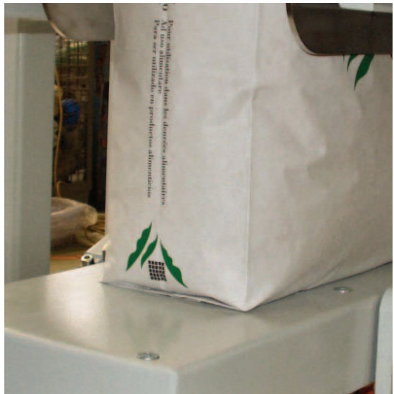
Perfect bag shape due to the use of vibrators
