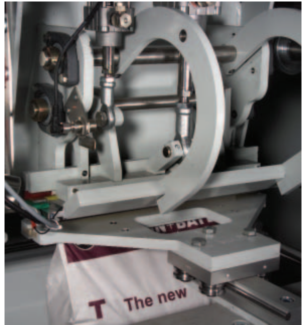
Bag closing and hot melt activation
