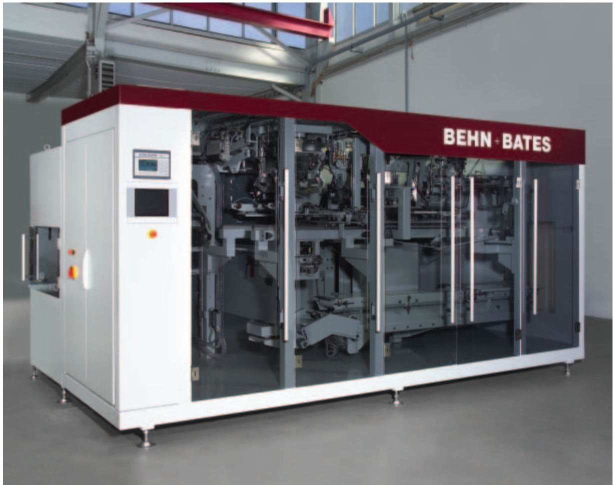
TOPLINE packing system with lateral empty bag magazine
